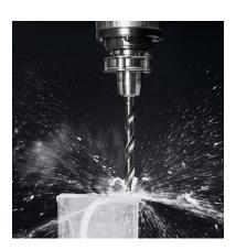
The switch to the new emulsifier technology of Multan 71-2 eliminates the problem of bacterial growth in metal-cutting fluids, without any need for later addition of bactericides.
